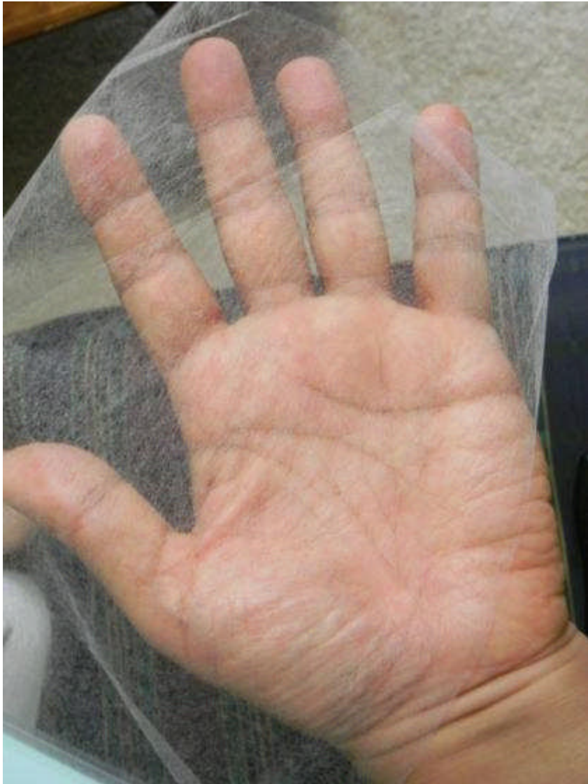
2 GSM polyolefin nonwoven (Hirose Paper)
